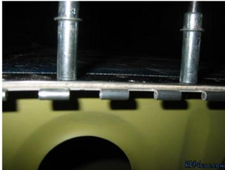
And the test fit. If the hinge pins don't easily go through the eyelets of the hinge, there are a few tricks:
