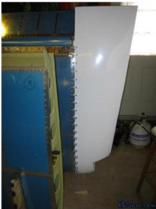
10) Permanently attach the wing side of the hinge to the wing. I dimpled the holes in the skin and countersunk the fiberglass flange from the wingtip.
