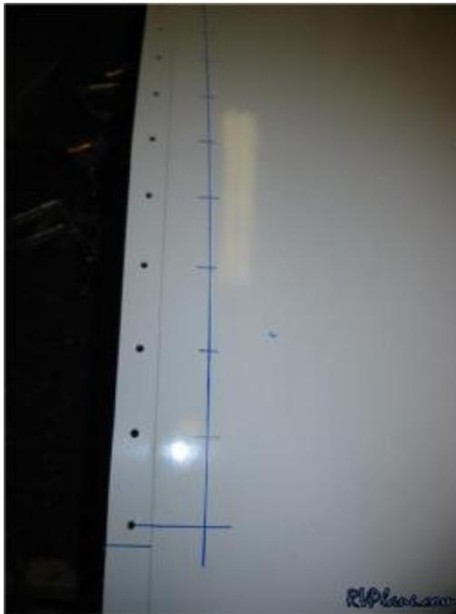
7) Using the marks made in the previous step, I backdrilled the P3 hinge.
